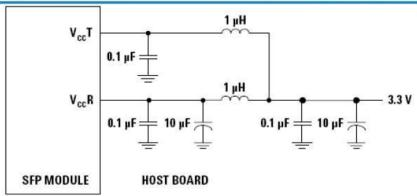
Note: Inductors with DC resistance of less than  $1\Omega$  should be used in order to maintain the required voltage at the SFP input pin with 3.3V supply voltage. When the recommended supply filtering network is used, hot plugging of the SFP transceiver module will result in an inrush current of no more than 30 mA greater than the steady state value.
