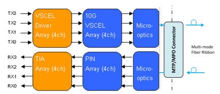
Figure 1: QSFP Transceiver Block Diagram
